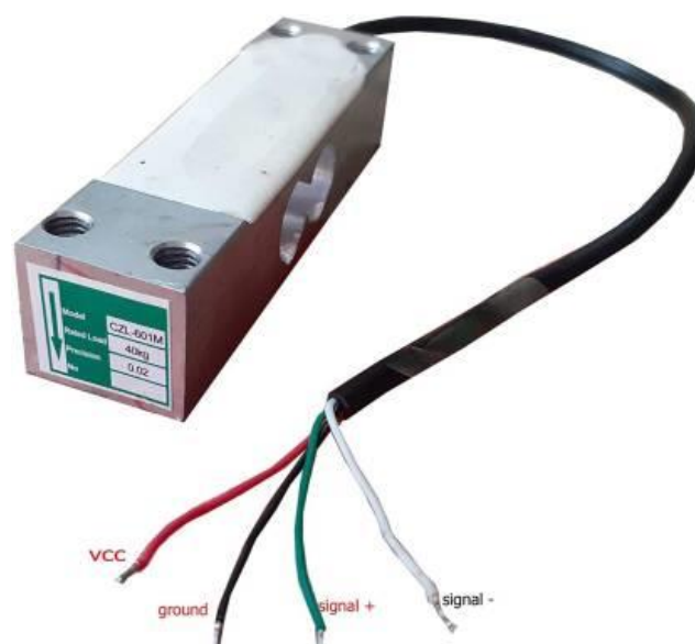
Fig 5.4 Load cell 40 KG
