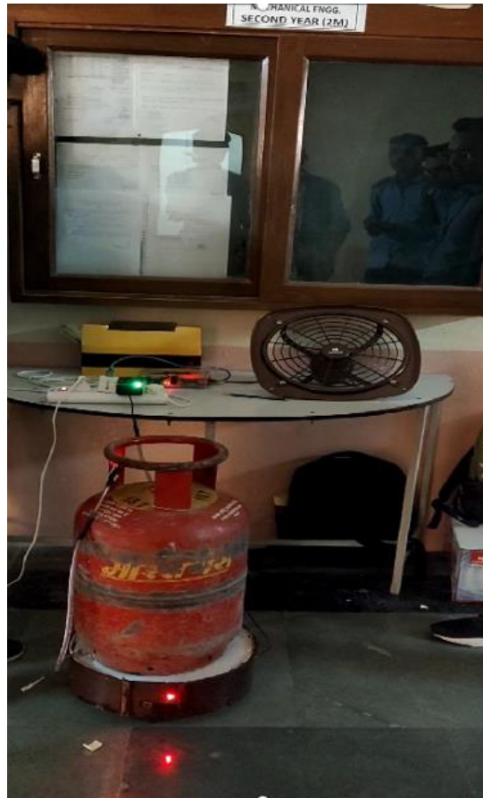
Fig 8.6 Cylinder 10 % Red LED & the exhaust on gas leaked detected.
